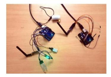
The Smart Farming System combines hardware and software components. Embedded systems are used in the hard ware and the software is creating dosing the Arduino IDE. Temperature and humidity sensors are among the sensors used. The data gathered by the sensors is for awarded to the server. UNO Arduino It is then relayed to a receiver through a transmitter.
